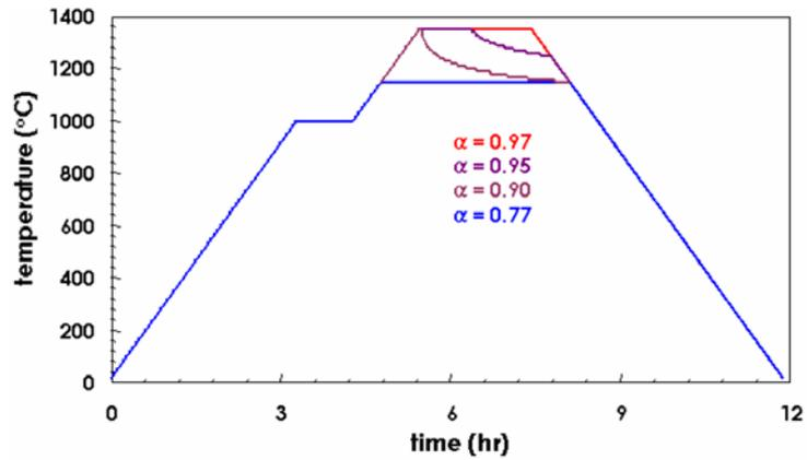
(b) corresponding sintering cycle
