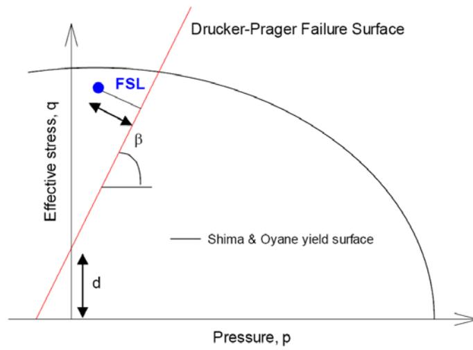
Figure 1. Definition of failure separation length (FSL) based on Shima and Oyane yield model and Drucker-Prager failure surface.
