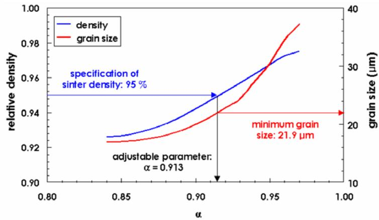
(a) sintered density and the corresponding minimum grain size
