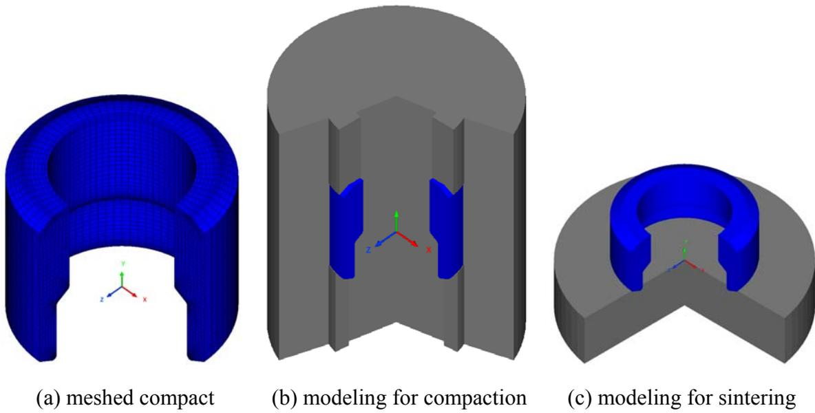
Figure 3. Example modeling and mesh generation example showing the simulation of compaction and sintering for an oxygen sensor housing; (a) mesh generation for the compact, (b) modeling of punches and dies during compaction for the press simulation, and (c) modeling of compact in contact with the substrate during sintering simulation.
