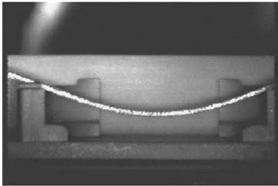
(a) in situ bending test
