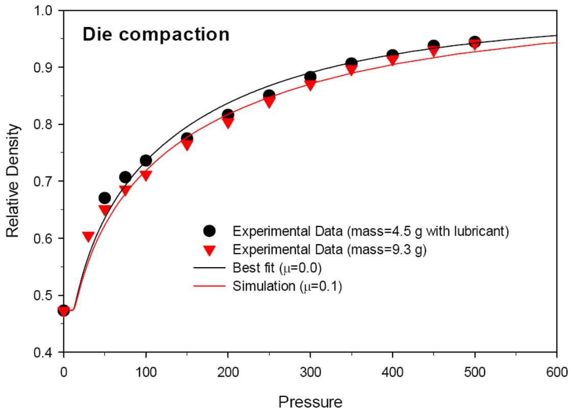
Figure 4. An example compaction curve for a iron-based powder, showing the relative density model results versus compaction pressure in MPa with no friction and with a friction coefficient of 0.1 for two compact samples [24].
