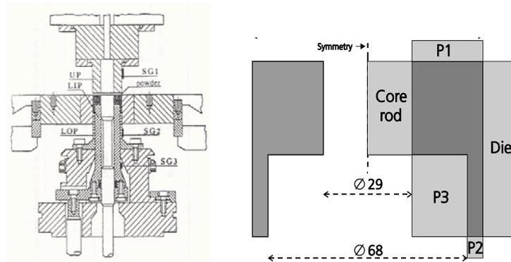
(a) compaction tool set and analysis domain
