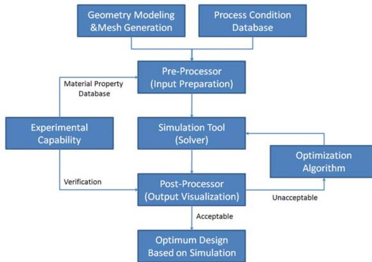
Figure 2. Typical procedure for computer simulation for press and sinter process.
