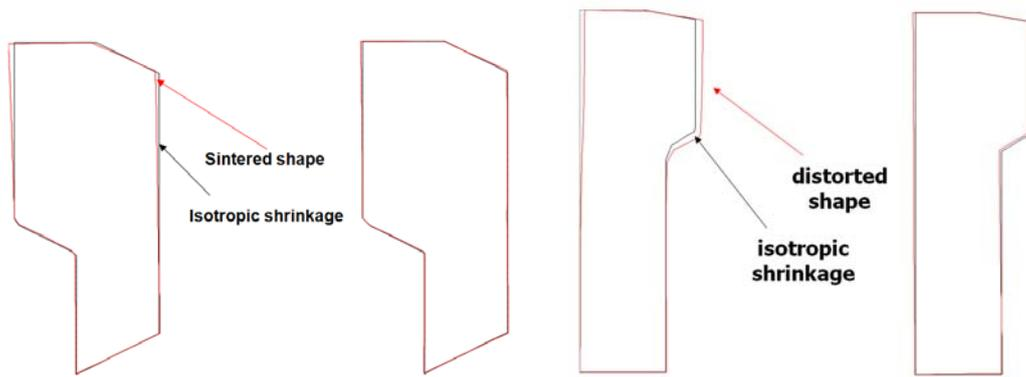
(a) initial and optimum holder designs      (b) initial and optimum sleeve designs
